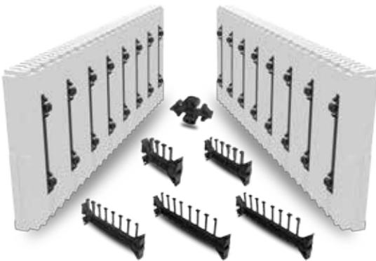
The BuildLock Knockdown ICF System is a high performance knockdown insulating concrete form (ICF) wall system with all of the same features of BuildBlock ICFs. It is comprised of two separate 2.5-inch Expanded Polystyrene (EPS) panels which are connected by strong, high-density plastic webs on 6-inch centers. BuildLock is the strongest knockdown product on the market today.
